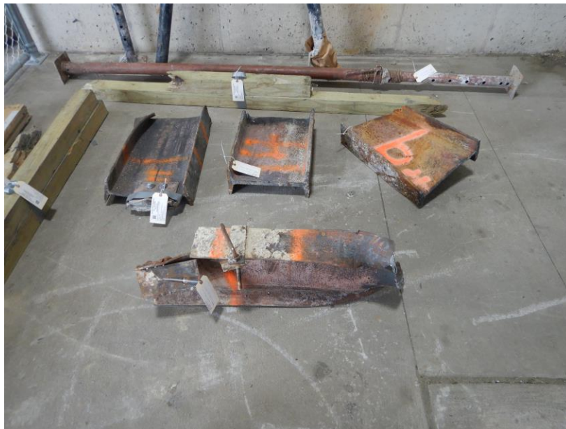
Appendix D - Photograph 2: Exemplar steel beam components.
